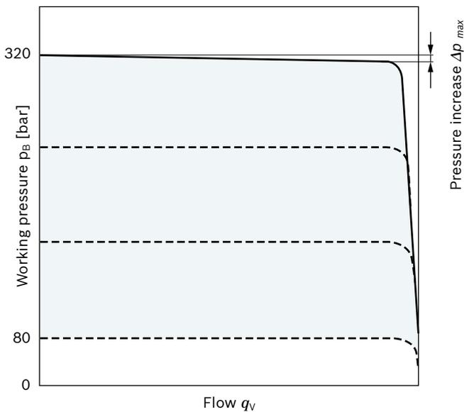
Characteristic curve valid for  $n_1 = 1500$  rpm and  $t_{\text{fluid}} = 50$  °C.
