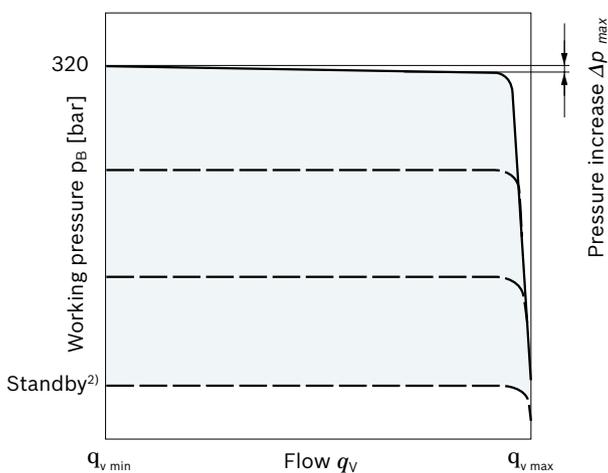
Characteristic curve valid for  $n_1 = 1500$  rpm and  $t_{\text{fluid}} = 50$  °C.
