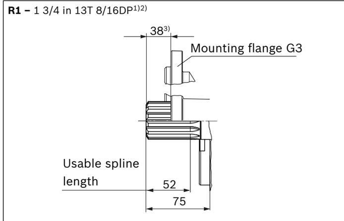
▼ **Splined shaft SAE J744**
